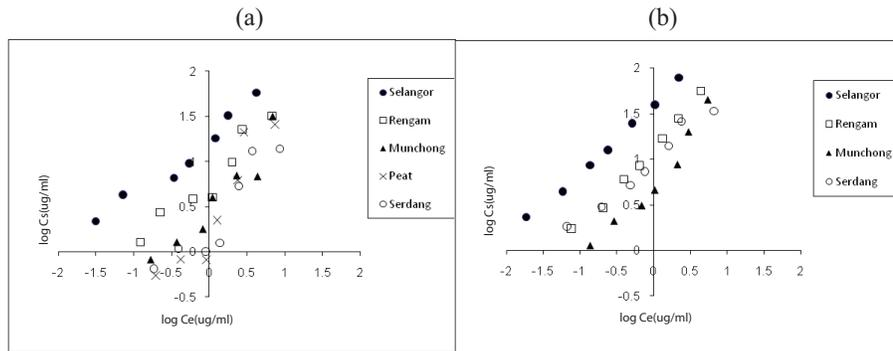
Fig. 3: Log-transformed Freundlich sorption isotherms of GLUF in (a) topsoil (0-15cm) and (b) subsoil (15-30cm) for the four soils
