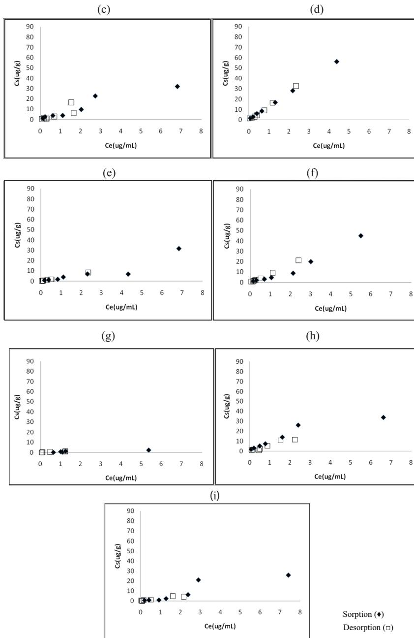
Fig. 4: Sorption and desorption isotherm of GLUF in topsoil (0-15cm) and subsoil (15-30cm) of (a) Selangor-topsoil, (b) Selangor-subsoil, (c) Rengam-topsoil, (d) Rengam-subsoil, (e) Munchong-topsoil, (f) Munchong-subsoil, (g) Serdang-topsoil, (h) Serdang-subsoil series soil and (i) peat
