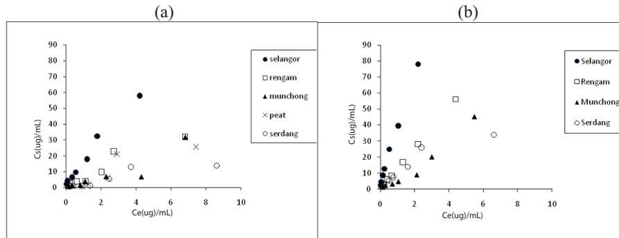
Fig. 2: Linear sorption isotherms of GLUF in (a) topsoil (0-15cm) and (b) subsoil (15-30cm) for the four soils.
